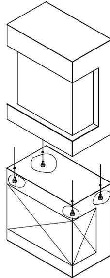
2. Unscrew the rear screws and remove the back steel panel
