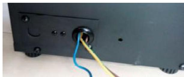
3. Replace the steel plate and screws.
