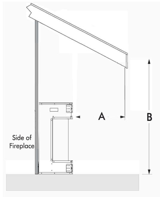
The overhang (A) must extend at least 1/2 the roof-line height (B). Height is measured from the base of the fireplace.
