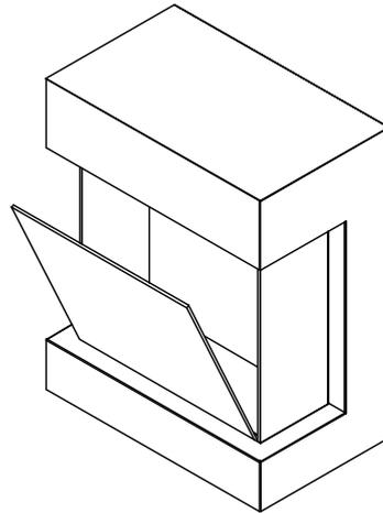
STEP 4: After finishing decoration, re-install the front glass panel using the securing screws removed in step 2.
