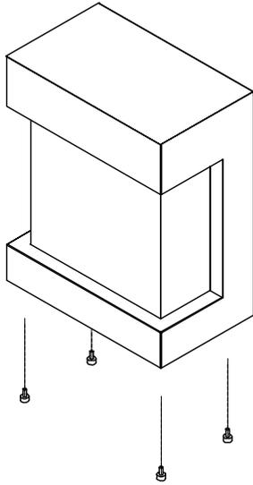
3. Place the unit on the CUBE-BASE-SPEAKER and screw in the adjustable feet, fixing the unit and the speaker box.
