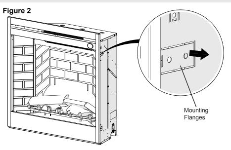
There are two mounting flanges located on each side of the fireplace insert. From the inside of the unit, bend tabs outward and mount to the inside of the framing using suitable hardware.
