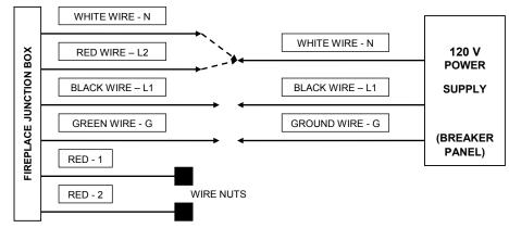
IMPORTANT: The unit is factory configured for 208/240V operation.
