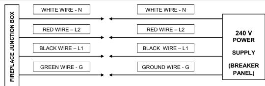
**IMPORTANT:** The unit is factory configured for 208/240V operation.
