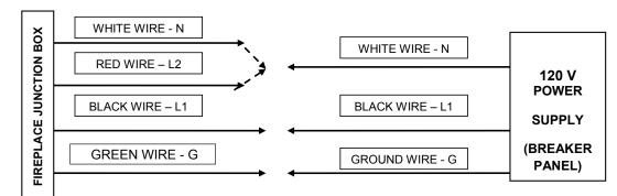
**IMPORTANT:** The unit is factory configured for 208/240V operation.
