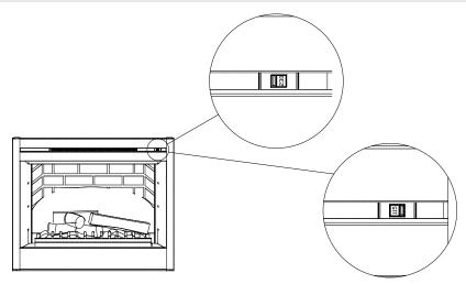
**IMPORTANT:** Ensure that the incoming power supply voltage matches the setting of the voltage selector switch.
