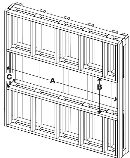
**CAUTION:** This fireplace is NOT load-bearing. Ensure the opening for the fireplace is framed in such a way that the weight of the building materials will not create pressure on the top of the fireplace.
