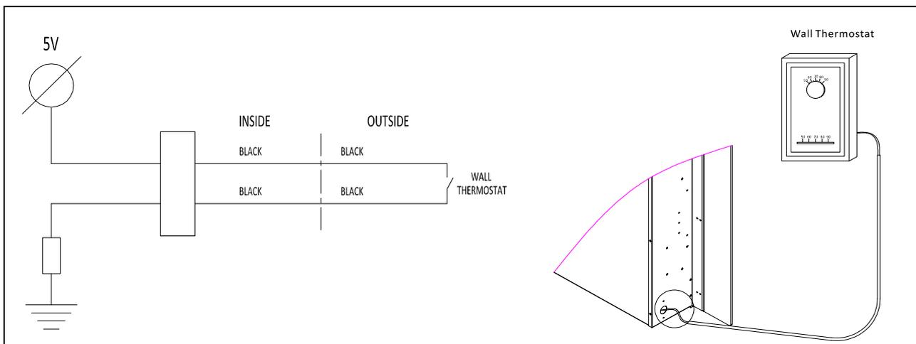
**NOTE: THE WALL THERM OSTAT WILL WORK ONLY WHEN THE HEATER IS SET TO TEM P. SETTING PLEASE REFER TO THE M ANUAL CONTROL AND THE REM OTE CONTROL**
