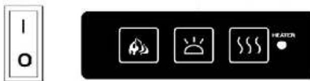
1. The main power ON/ OFF switch in position O, the fireplace is OFF.
