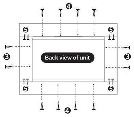
For ease of install, lay fireplace face down on a cloth (soft) surface, when installing trim pieces.
