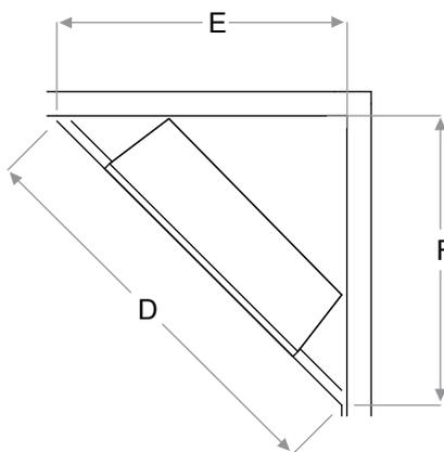
**NOTE:** The materials used for the finished surround must be cut to precise dimensions as the 1/2" (1.3 cm) self trimming flange is only to create a finished appearance.
