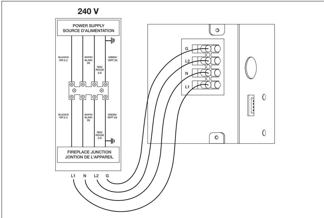
1. Insert Green or bare copper wire to the designated G Terminal. Tighten the screw.
